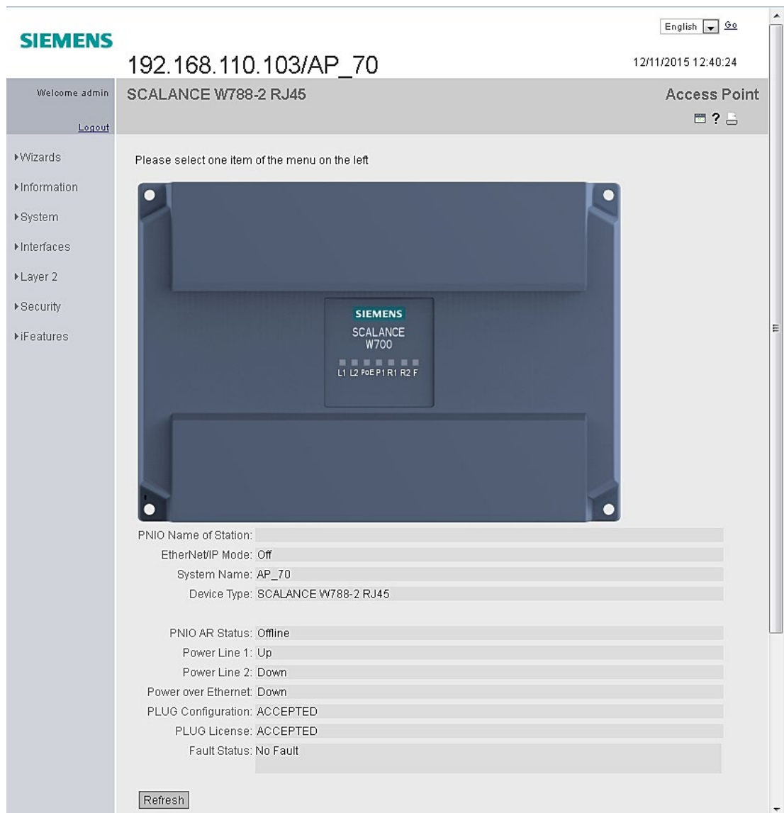
Figure 4-1 Web Based Management based on the example of configuring a W788 access point
